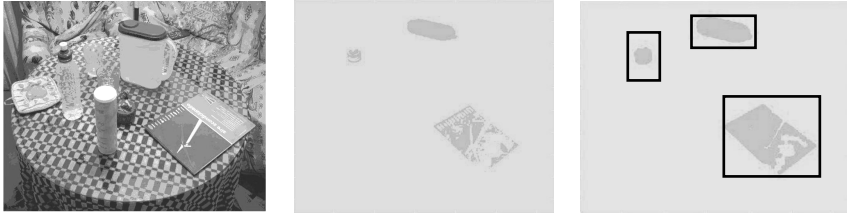
Fig. 1. Different processing stages: original image (left), the pixel segmentation (centre) and the image after pixel dilatation and erosion process (right) are presented. Object detection is marked by a black square indicating the presence of the target object.
